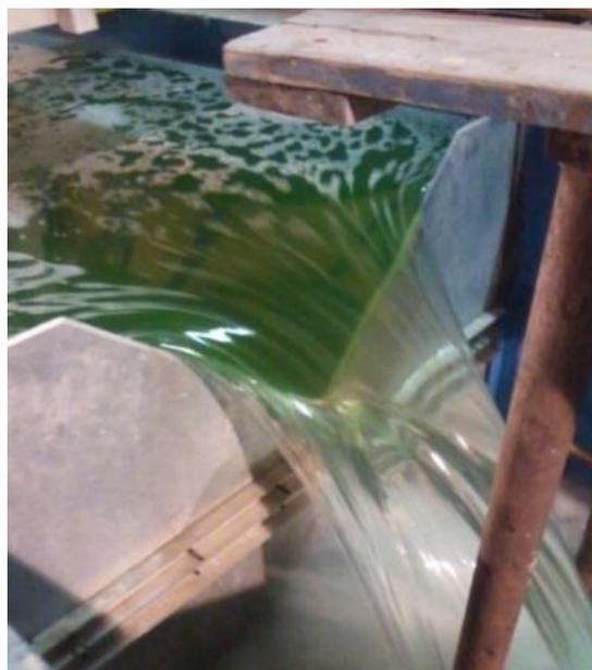
**Figura 31: Vertedero triangular calibrado**
