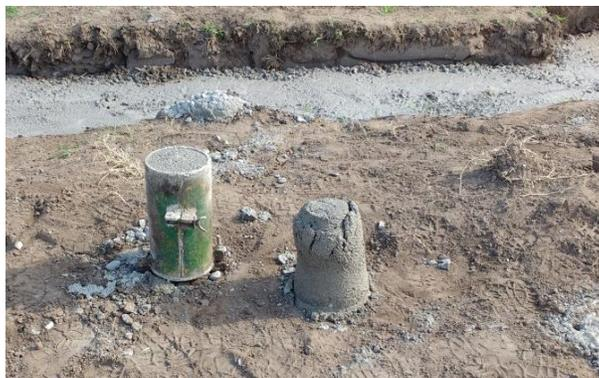
Figura 3.4.18 Cono de Abrams defectuoso
