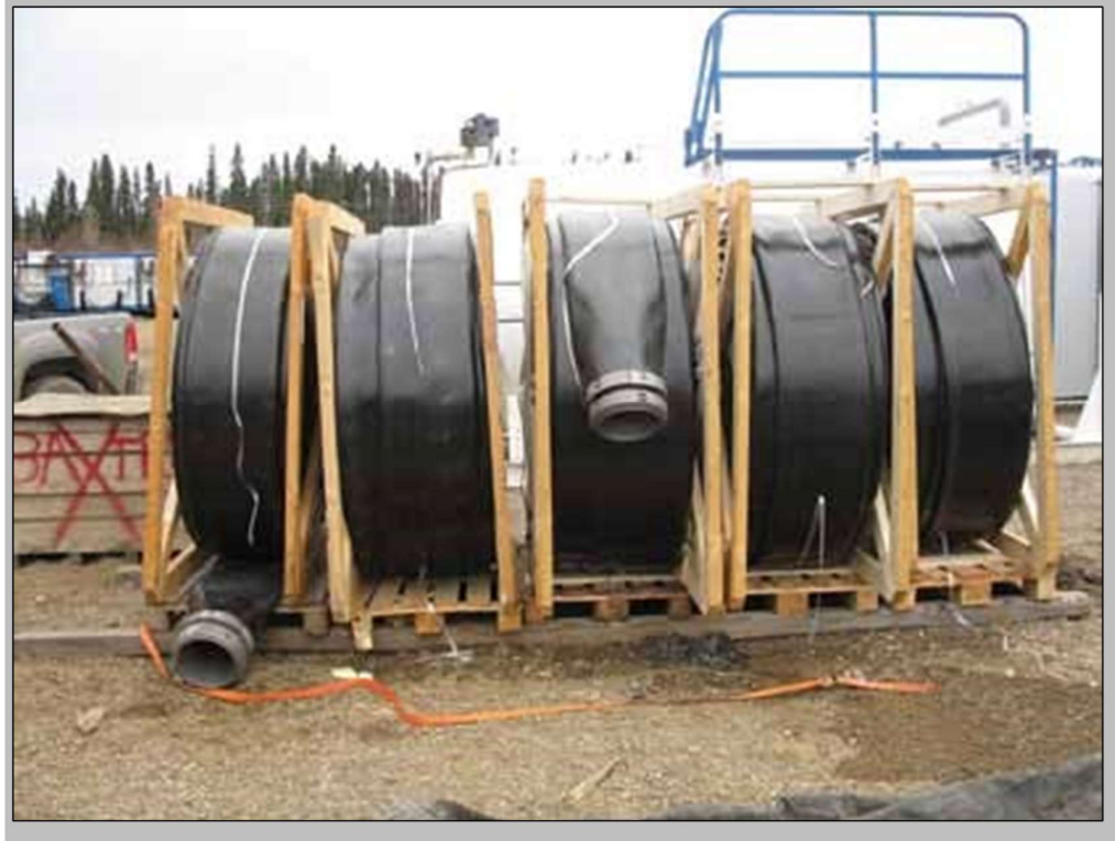
1,000m x 10" Mine flex Delivered into the field
