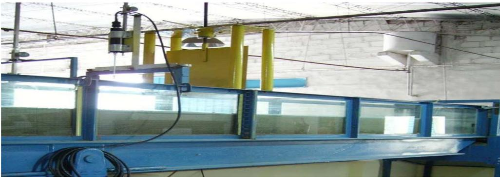
Figura 26 – Modelo 2D – Canal Experimental
