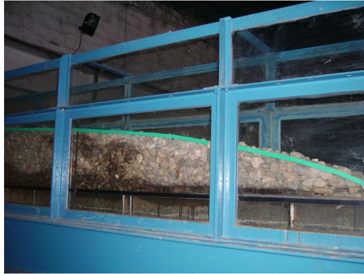
Figura 4-6 Playa absorbente instalada
