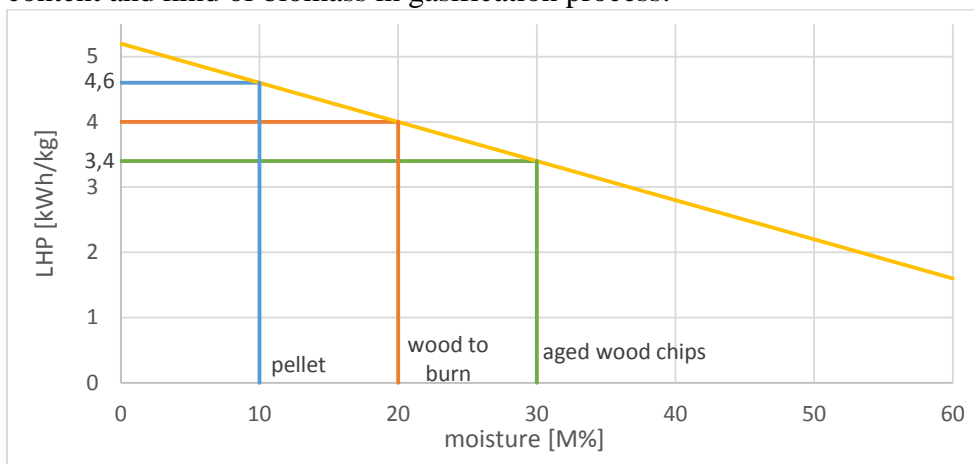
Fig. 3: Trend of LHP of woody matters in function of contents [1]
