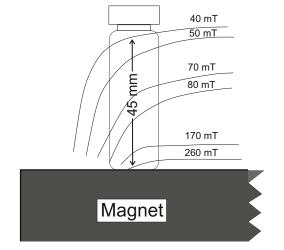
**Fig. 1** Sketch of the permanent magnet and the lines (surfaces) of constant magnetic field strength, as indicated, which have been previously mapped out using a Hall probe. The sample was placed always at the same marked position near the edge of the magnet. The resulting gradient of the magnetic field is roughly 5 T/m.
