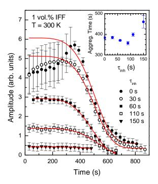
**Fig. 5** Dependence on time of the amplitude (symbols) of the real part of the FID signal within the first stage of its evolution for different dwelling times  $\tau_{inh}$  in the magnetic field gradient. Red curves correspond to a fit through the amplitude data points using Eq. (11). The inset shows the values of the characteristic aggregation time  $\tau_{agg}$  in a homogeneous field obtained from the fit as a function of the time  $\tau_{inh}$  the IFF dwelled in the field gradient.
