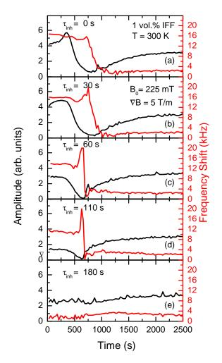
**Fig. 3** Time evolution of the amplitude (black line) and frequency shift (red curve) of the real part of the FID signal measured for the IFF sample after different dwelling times  $\tau_{inh}$  of (a) 0 s, (b) 30 s, (c) 60 s, (d) 110 s, and (e) 180 s in an external magnetic field gradient of roughly 5 T/m.
