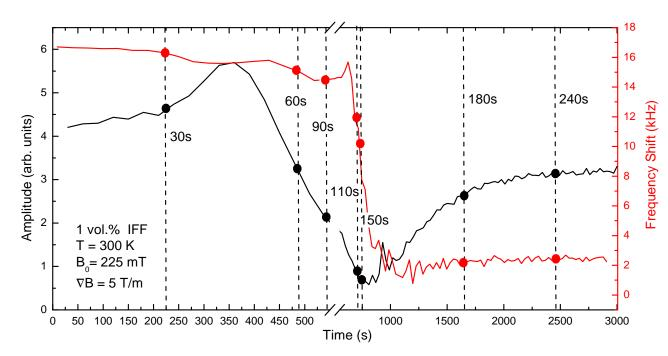
Fig. 7 Time evolution of the amplitude (black curve) and frequency shift (red curve) of the main NMR peak measured for the pristine IFF sample ( $\tau_{inh} = 0$ ) every 30 s for times up to 3000 s. The black and red closed circles correspond to the amplitude and frequency at the beginning of a similar measurement series but performed after the IFF was sitting a time  $\tau_{inh}$  in the external magnetic field gradient, as indicated.
