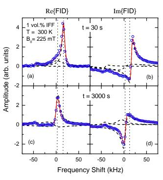
**Fig. 2** Real and the imaginary part of the Fourier transformed FID signal (open blue symbols) at two different times for the pristine sample, i.e., without having experienced any field gradient, (a,b) at the beginning of the measurement and (c,d) after 3000 s. The solid red lines correspond to the total fitting function, whereas the dashed black lines represent each of the three resonances composing the full signal.
