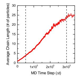
**Fig. 4** Molecular dynamics results corresponding to the time evolution of the the average chain length of IFF particles in the presence of a homogeneous magnetic field.
