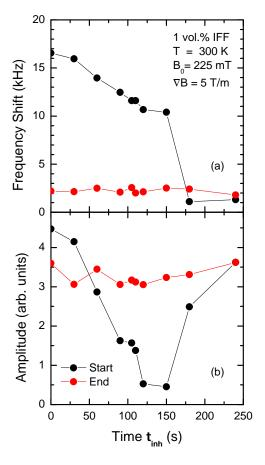
**Fig. 6** (a) Frequency shift and (b) amplitude of the main NMR peak of the ionic ferrofluid at the beginning ( $\approx 30$  s, black symbols) and the end ( $\approx 3000$  s, red symbols) of each measurement series as a function of the exposure time to the external magnetic field gradient.
