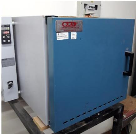
IMAGEN 16: HORNO ELECTRICO TIPO MUFFLA
