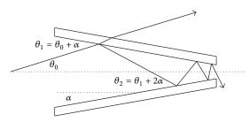
FIGURE 2: Schematic diagram of the radiation transport through the conical monocapillary.
