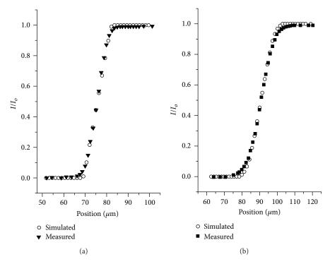
FIGURE 5: Measured and simulated vertical profile of the microbeam: (a) at 1 mm and (b) at 10 mm. In (a) the mean FWHM for the simulated beam is  $22.1 \,\mu$ m and the measurement gives  $22.3 \,\mu$ m. For (b) the mean FWHM for the simulated beam is  $34.5 \,\mu$ m and the measurement gives  $34.7 \,\mu$ m.
