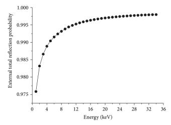
FIGURE 3: Probability of total reflection as function of energy, for photons at the third reflection with the largest incident angle in the total reflection regime. It was calculated through (4) taking  $\delta=2$  and the incident angles at each reflection equal to the total reflection angle.
