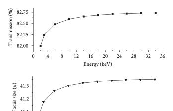
FIGURE 4: Percent transmission and focus size of the excitation channel lens at 15 mm from its output versus the incident energy. Here the focus size is represented by the FWHM of the transversal cross section of the emergent beam. It is given by product of  $\sigma_A$  by 2.35482.
