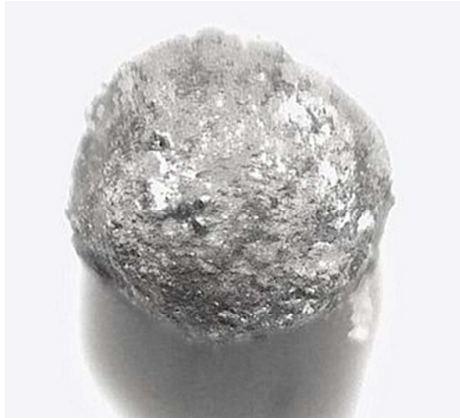
Figure 6: a) A photograph (Motic 40x) of a weathered bullet. b) Microphotography 1400x taken by a Lext 3D Laser microscope OLS 4000 Olympus of crust. 87x79mm (96 x 96 DPI)
