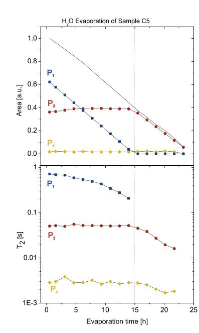
Water in highly crosslinked networks evaporates in steps from the bigger pores to the smaller ones. The evaporation steps are consecutive and start only when the previous pore is dry. Water adsorbed to the mesh is not removed at 25°C.
