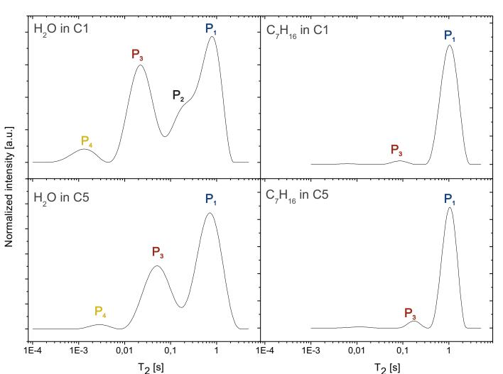
Heptane does not swell the matrix and the liquid molecules are mainly located in the macropores. A minor population is placed in the mesopores revealing that in the dry state the main contribution to the porosity of the polymer is given by the larger pore spaces.
