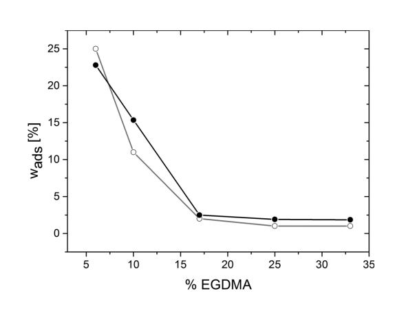
The percentage of water adsorbed by the network obtained by weighting methods can be compared with the areas under the relaxation time distributions corresponding to  $P_2$  plus  $P_4$ . The remarkable coincidence indicates that the assignment of  $T_2$  distribution to the swollen water is correct. It is worth to note that  $P_2$  can only be distinguished for water saturated samples C1 and C2, where the low percentage of crosslinker renders a soft network that is capable of swelling.
