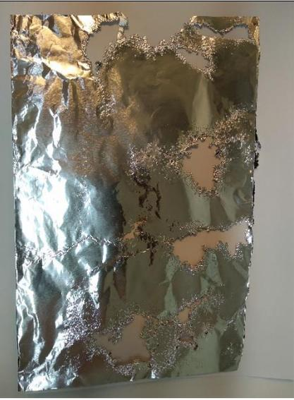
A photograph of a piece of crumpled aluminum foil. The surface is significantly more damaged than in the 3-minute test, with large areas of the foil missing, revealing a brownish, porous material underneath.                                                                                      |
