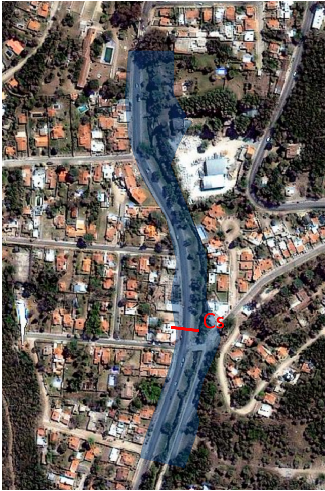
Fig. 4. Flooded area estimated using the HEC-RAS flood model calibrated with the LSPIV velocity measurement and the water level data in the section of interest (marked Cs). The peak discharge was estimated to be 290 \text{ m}^3/\text{s} .
