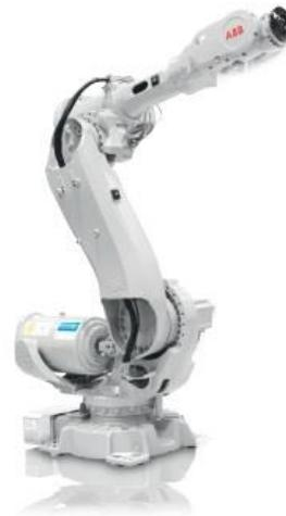
Upper arm extenders and different wrist modules allow customization to each process. As the robot can bend fully backwards, the working range is greatly extended allowing it to fit well into dense production lines. Typical application areas are material handling, machine tending and spot welding.
