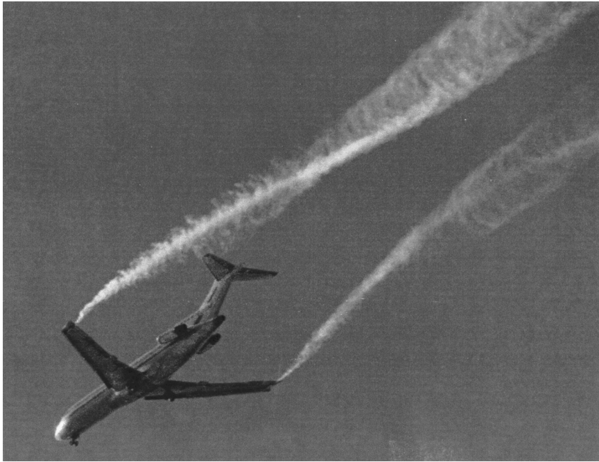
Figure 8.12 Flow visualization of the rollup of the trailing vortices behind an airplane (wing tip vortices made visible by ejecting smoke at the wing tips of a Boeing 727 airplane). (Courtesy of NASA.)
