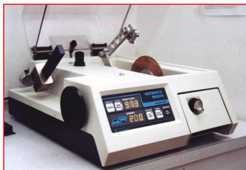
Figura 9: Micrótopo IsoMet® 1000, Buehler Co.
