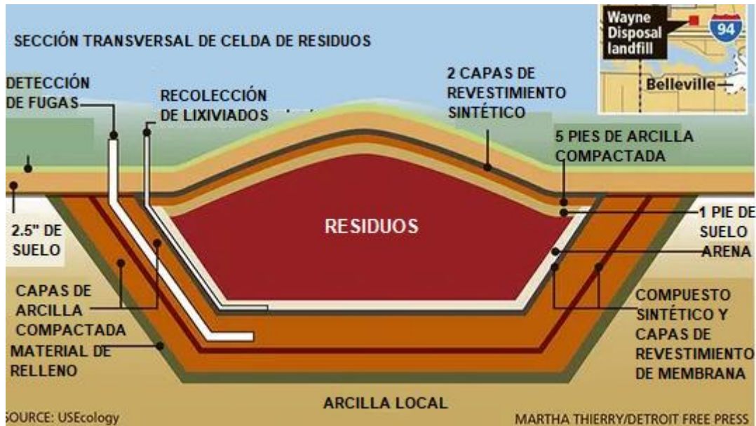
Figura 31: Relleno de seguridad (Recuperado de https://www.freep.com/story/news/local/michigan/2014/09/07/landfill-taking-radioactive-waste-has-history-of-violations-leaks-fires/15210857/ )
