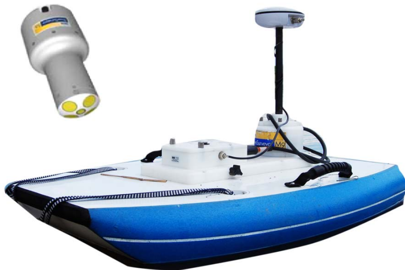
Figura 5.2: ADCP River Surveyor S5®. Fuente: www.sontek.com/riversurveyor-s5-m9.php
