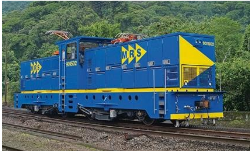
▪ Fig. 12. The most powerful rack locos in the world, built to operate the world's busiest mainline rack, the Serra incline in Brasil. Seven locos were built by Stadler in Switzerland in 2012. P Mahoney collection.
