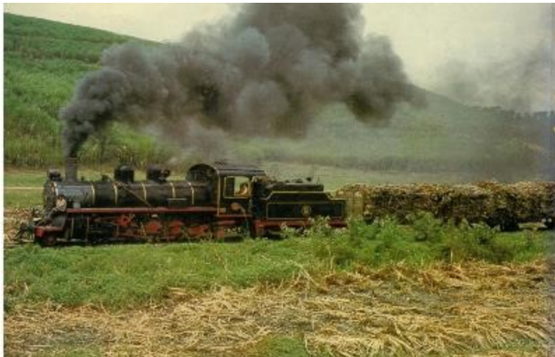
▪ Fig. 16. Industrial railways in South America. Sugar cane harvesting action on the plantation railway of Usina Santa Therezinha in Pernambuco State, Brazil. This 1973 scene shows great company pride in a beautifully maintained 2-8-2 type loco, of USA origin, hauling a train of freshly cut cane. (The loco identity is Alco 65540/1924) Photo: Roy Christian. P Mahoney collection.
