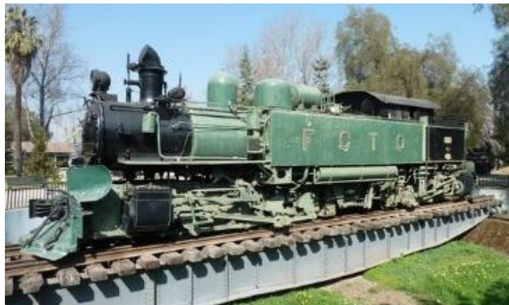
▪ Fig. 4: A specialised mountain railway loco. This hefty 90 tonne loco worked in Chile on the Transandine mainline railway linking Santiago and Buenos Aires. It is a 'rack loco' built by the Kitson Company in England in 1909. Toothed 'rack pinions' under the loco continuously engage with a central toothed 'rack rail' laid between the normal rails, to provide a very positive grip to climb and descend steep mountain grades. P Mahoney collection 1990.
