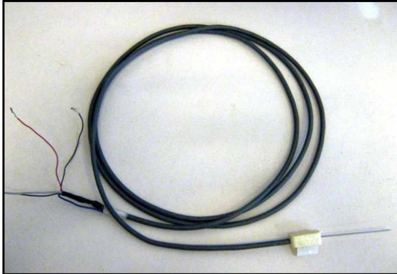
Figura 3.5: Sensor de aguja simple EAST-30.
