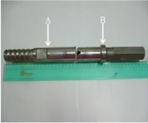
Figure 2. Broken shank adapter.
