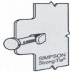
Double Shear Nailing Side View U.S. Patent 4,291,996
