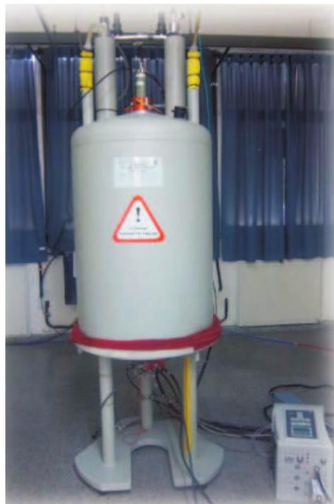
FIGURA 3.1: Imán superconductor Bruker de 7 T.
